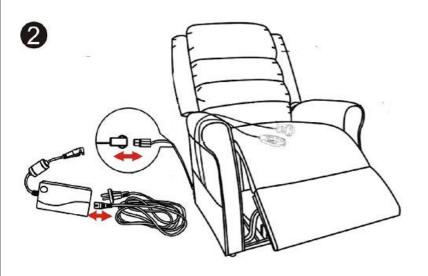
2) Connect the Lift and Recline supply cable pins. Fit the pins properly in the manner shown in the image. Do not force them, they only have one correct position.
