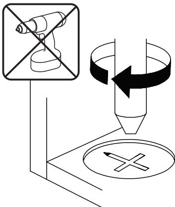
**EN**\_Turn cam lock clockwise to tighten.
