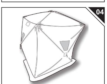
Lifting the roof of shelter up, pull outward on the center hub of one of the walls. Continue around the entire shelter, pulling each wall hub until all of walls are set up.
