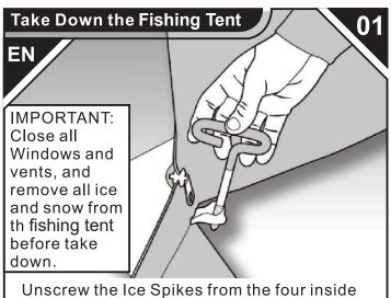
Unscrew the Ice Spikes from the four inside corners and remove all tie down(s) from the outside wall(s). Place all Ice spikes and straps in the supplied pouch and store in the case pocket.
