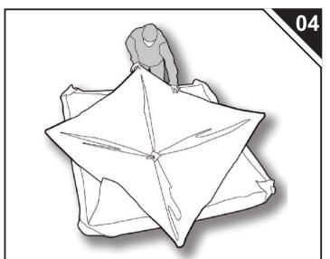
Once the unit is laying flat, lift each of the corners together and stand the folded unit with all of the hubs facing down.
