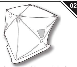
Push in firmly on one of the center hubs of the outside walls until it collapses inward. Continue around the outside of the fishing tent collapsing all of the remaining walls until the unit lays flat.
