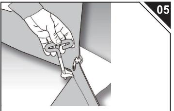
Position the Fishing tent over fishing hole in the ice, and secure each inside corner of shelter to ice by screwing one of the included ice spikes through the' small loop into ice. Push down while twisting ice spike until it gets started, and then twist the spike until it holds fast.
