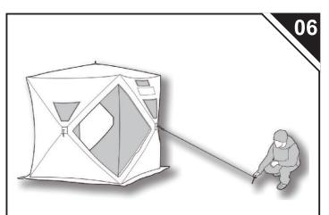
Find the side of the Fishing tent that faces into the wind and attach one of the provided straps to the center hubs of that wall. Stretch the strap into the wind and with the remaining Ice Spike(s), secure the strap to the ice.
