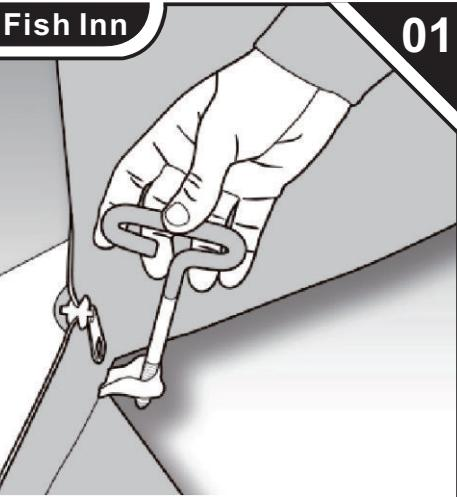
Unscrew the Ice Spikes from the four inside corners and remove all tie down(s) from the outside wall(s). Place all Ice spikes and straps in the supplied pouch and store in the case pocket.
