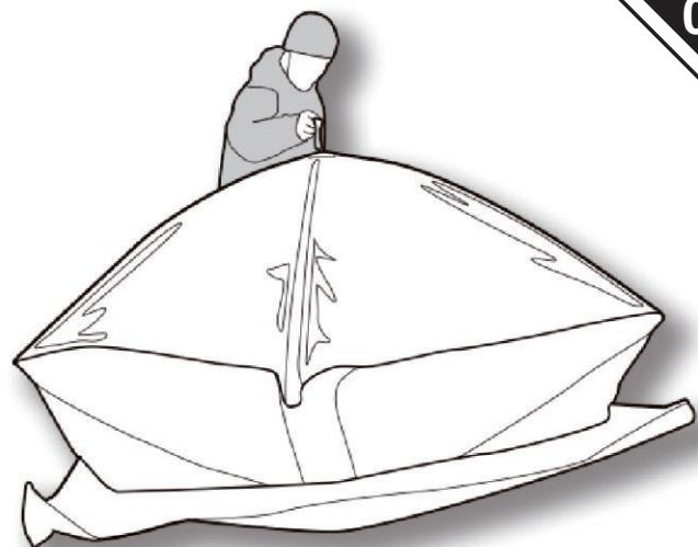
Firmly push down on the the center hub(s) of the roof with the palm of your hand until the roof flattens down onto the sides.
