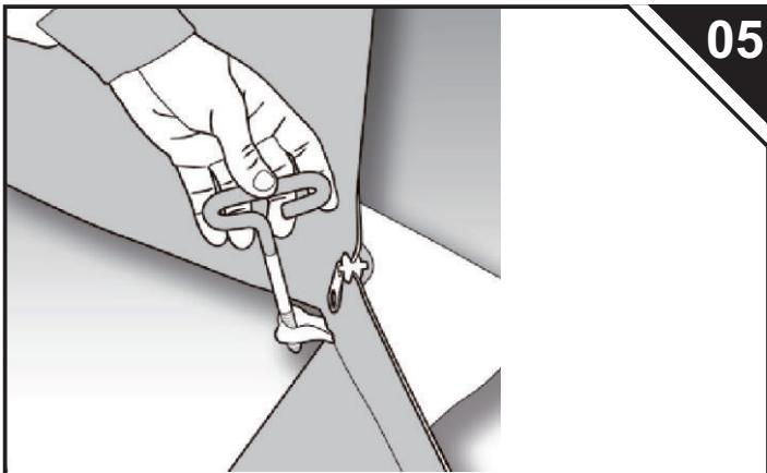
Position the Fish Inn over fishing hole in the ice, and secure each inside corner of shelter to ice by screwing one of the included ice spikes through the small loop into ice. Push down while twisting ice spike until it gets started, and then twist the spike until it holds fast.
