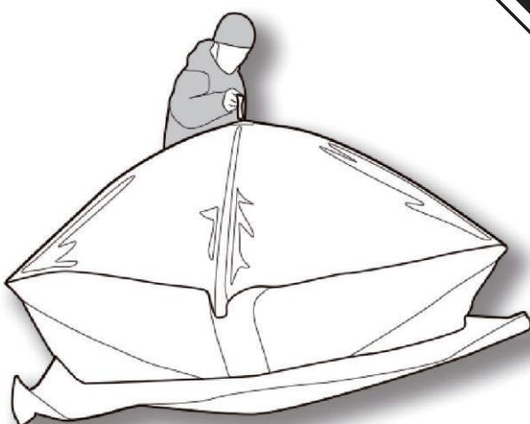
Firmly pull up on the strap in the center hub of the roof until it pops up. Twist the roof slightly so corners of top and bottom line up.
