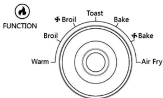
**Warm:** Turn the function knob to Warm and turn the temperature knob to Warm. Then turn the Oven Timer knob to the desired warming time to start the oven and begin warming. The power light will illuminate. The timer will ring once when the cycle is complete and the oven will power off when the time expires.
