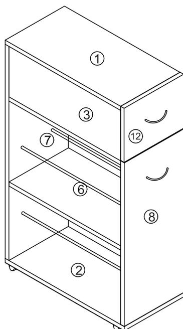
**EN\_** Be careful to push in the board when the both sides slide way been aligned.
