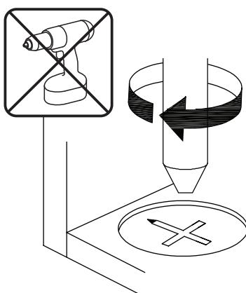
**EN**\_Turn cam lock clockwise to tighten.
