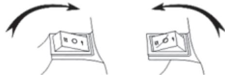
Apply the wrench to the wheel nut, then press the upper side of the switch (marked 'L'). The nut will loosen . Press the upper side of the switch (marked 'T') and the nut will tighten.
