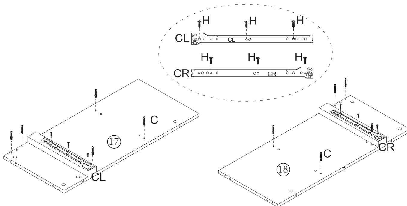
**EN** Please find the exact hole for installation, otherwise it will be misaligned. The screws on the drawer slide must be leveled, otherwise it will affect the smoothness of the drawer.
