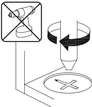
**EN\_Turn cam lock clockwise to tighten.**
