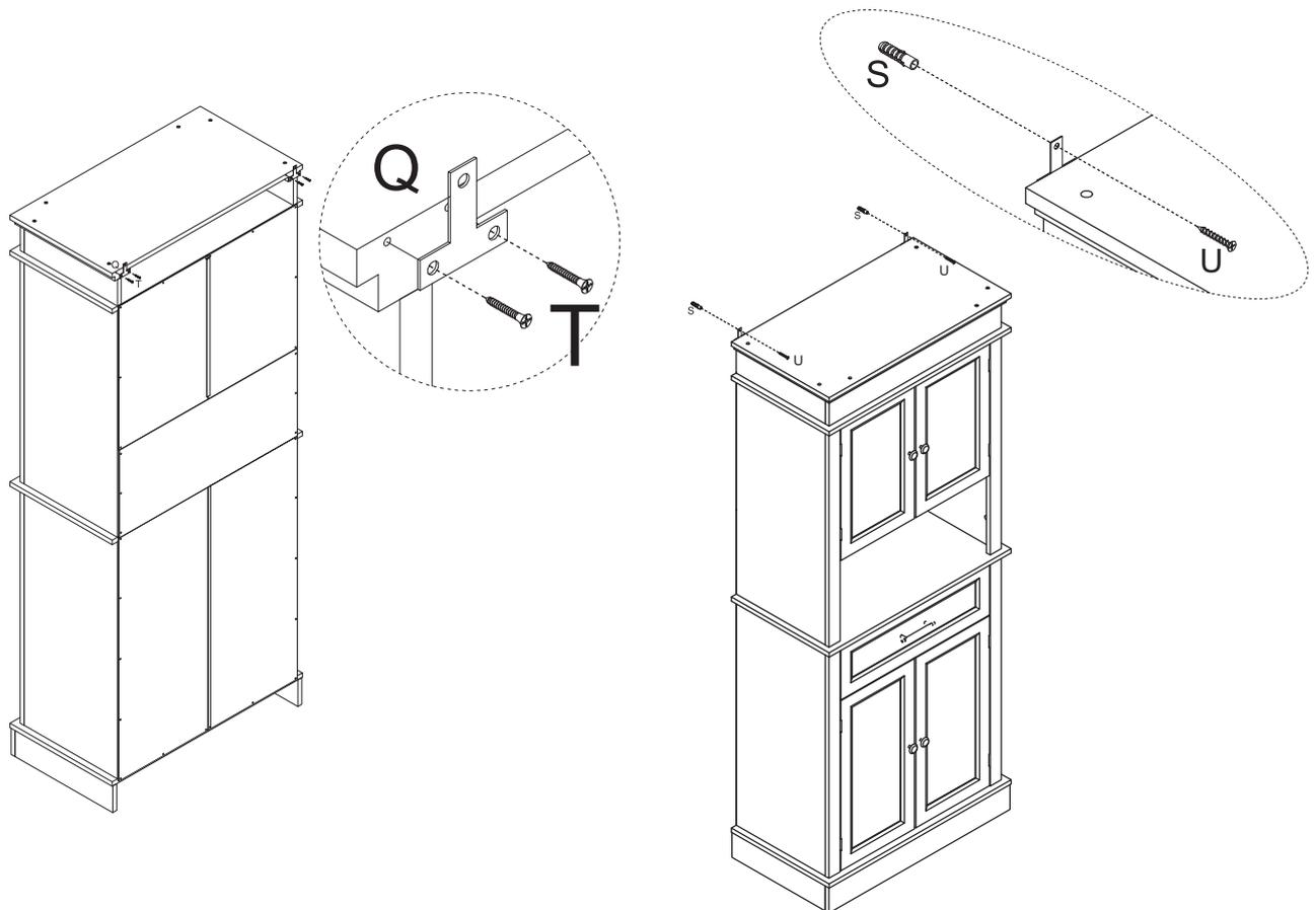
**EN** If it is a solid wall, please use expansion and self-tapping screws, if it is a wooden wall, only use self-tapping screws, please do not overtighten the screws
