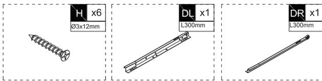
**EN** Please find the exact hole for installation, otherwise it will be misaligned. The screws on the drawer slide must be leveled, otherwise it will affect the smoothness of the drawer.
