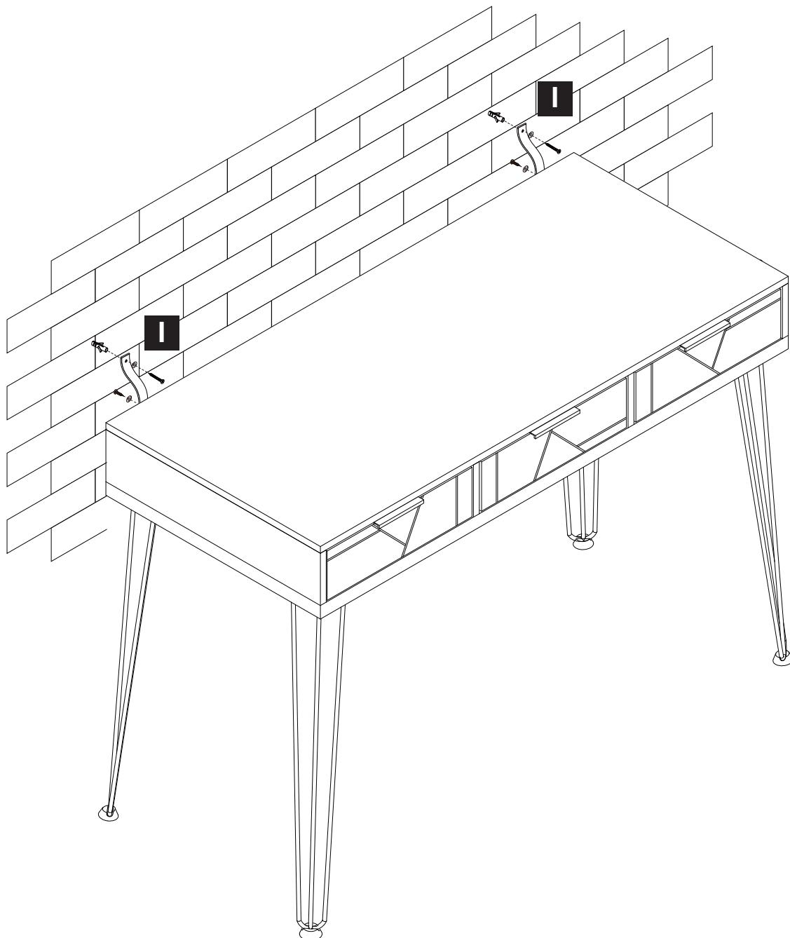
**EN** If it is a solid wall, please use expansion and self-tapping screws, if it is a wooden wall, only use self-tapping screws, please do not overtighten the screws
