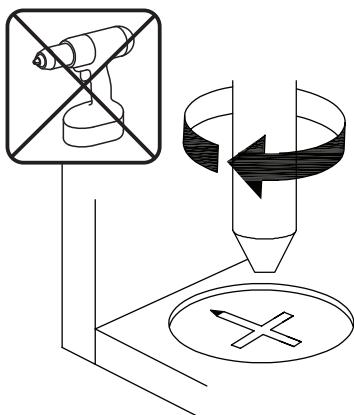
**EN**\_Turn cam lock clockwise to tighten.
