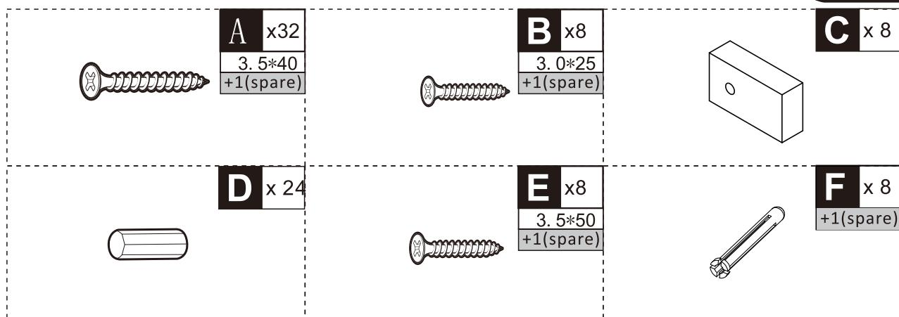
**EN** If it is a solid wall, please use expansion and self-tapping screws, if it is a wooden wall, only use self-tapping screws, please do not overtighten the screws
