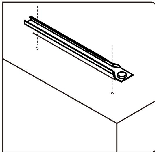
**EN** Please find the exact hole for installation, otherwise it will be misaligned. The screws on the drawer slide must be leveled, otherwise it will affect the smoothness of the drawer.
