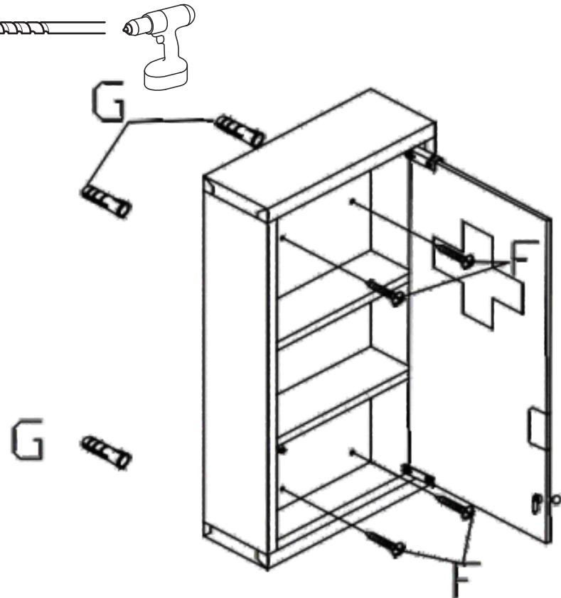
**EN** If it is a solid wall, please use expansion and self-tapping screws, if it is a wooden wall, only use self-tapping screws, please do not overtighten the screws
