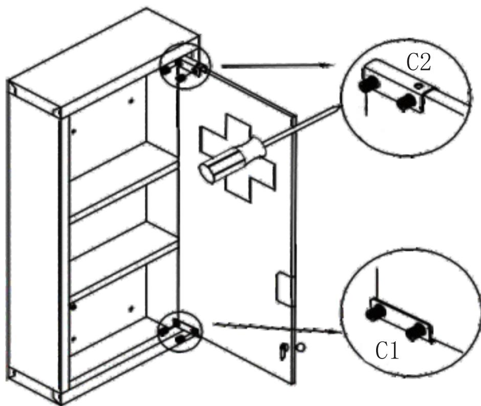
**EN** When closing the door, if there is a gap, please adjust the fixing position of the metal parts C1, C2 and the door appropriately.
