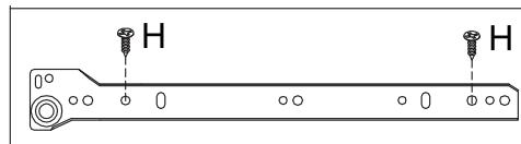
**EN** Please find the exact hole for installation, otherwise it will be misaligned. The screws on the drawer slide must be leveled , otherwise it will affect the smoothness of the d rawer.
