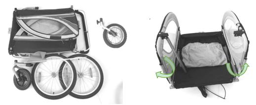
Swing the crossbar upward into position across the top between the side panels and route it through the loops at the top of seat. Insert the crossbar into the upper sleeve and lock with the safety pin.
