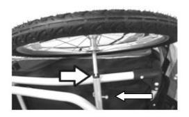
To remove the wheels lift the trailer and remove the safety hook.
