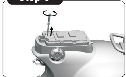
8. Loosen the screw with a screwdriver (not included).
