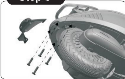
3. Place the rear fender over the location in the rear of body, tighten by four M4X14 screws with a screwdriver (not included).
