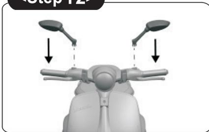
12. Insert the rear-view mirror into the hole of the handle bar, be certain the rear-view mirrors are completely fixed.
