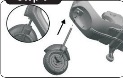
5. Insert the front wheel stick into the hole of the body, make sure the right position.
