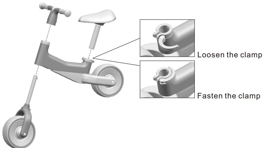
1. Insert the front wheel set from the bottom hole of the body as shown in the figure, then fix the handle bar with front wheel.
