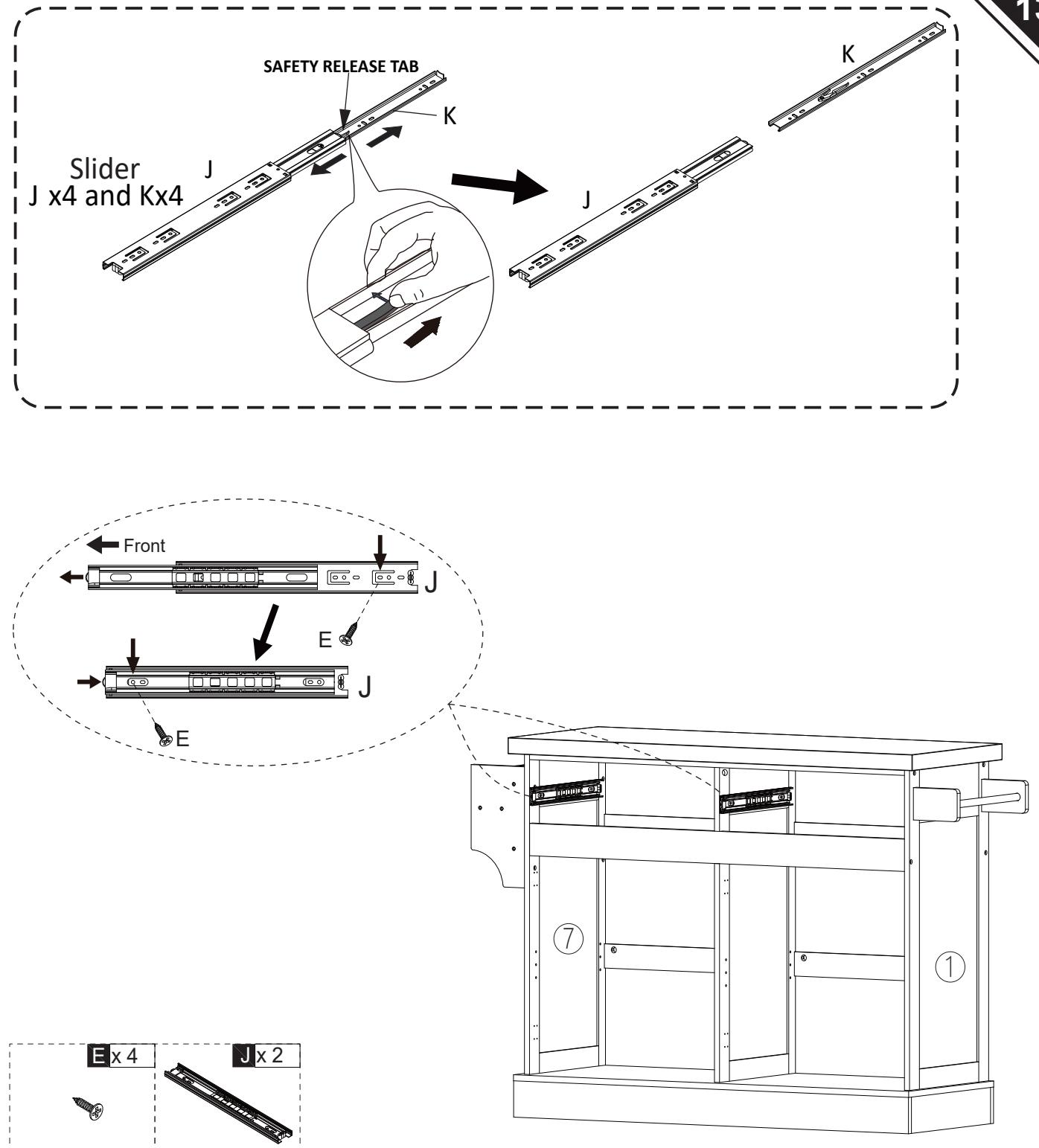
**EN** Please find the exact hole for installation, otherwise it will be misaligned. The screws on the drawer slide must be leveled , otherwise it will affect the smoothness of the d rawer.
