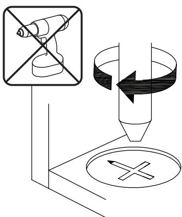
**EN**\_Turn cam lock clockwise to tighten.
