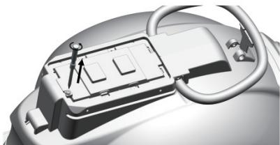
9. Loosen the screw with a screwdriver (not included).
