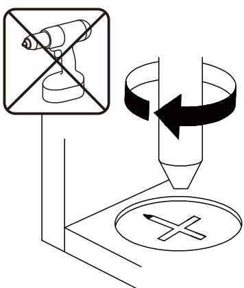
**EN**\_Turn cam lock clockwise to tighten.
