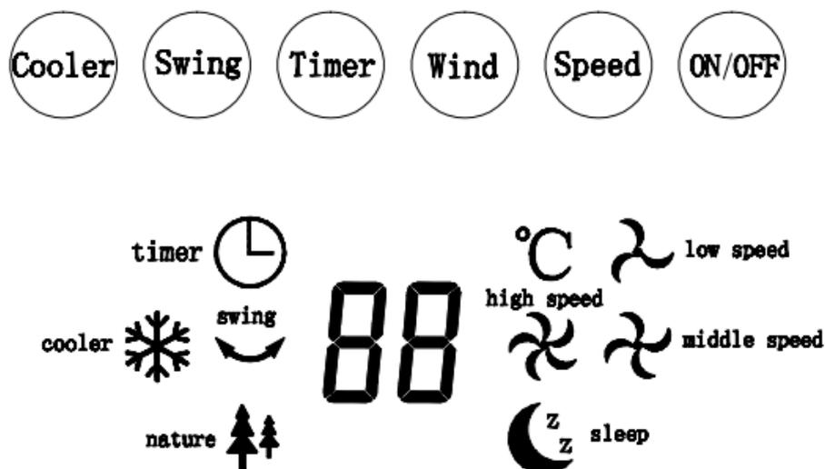
Insert plug to the electrical outlet. Press the “On-Off” button to switch the unit “On”. The LED indicator automatically shows the room temperature and shifts the fan to stand by position. The function of the unit can be controlled via on board control panel or by remote.
