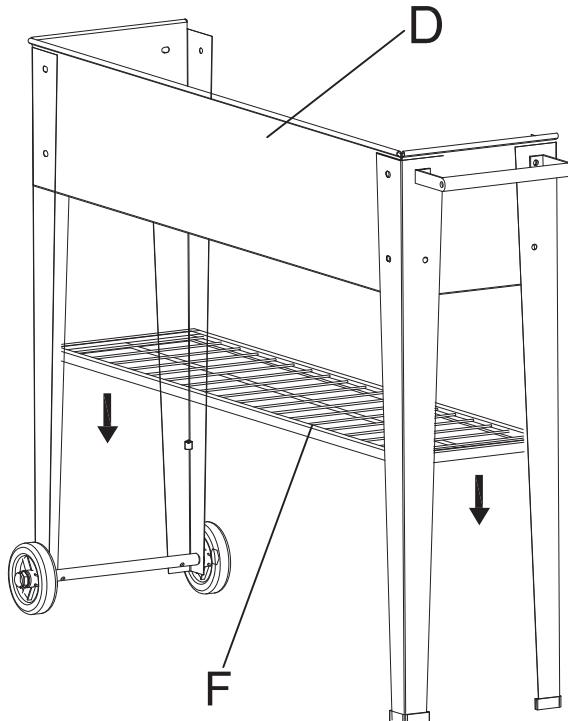
**EN\_NOTE:** The Legs should be on the outside of the planter with the ledge on the Side Panel facing in. Insert a bolt into each set of holes and loosely attach a nut onto the end of each one. Each corner of the Shelf (F) has a hook on it. Position the Shelf between the Planter Cart's legs and slide the hooks into the slots on the inside of each leg.
