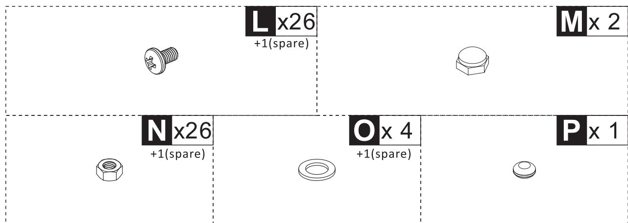
**EN** \_Do not confuse similar screws. Do not tighten bolts fully until all parts are connected!
