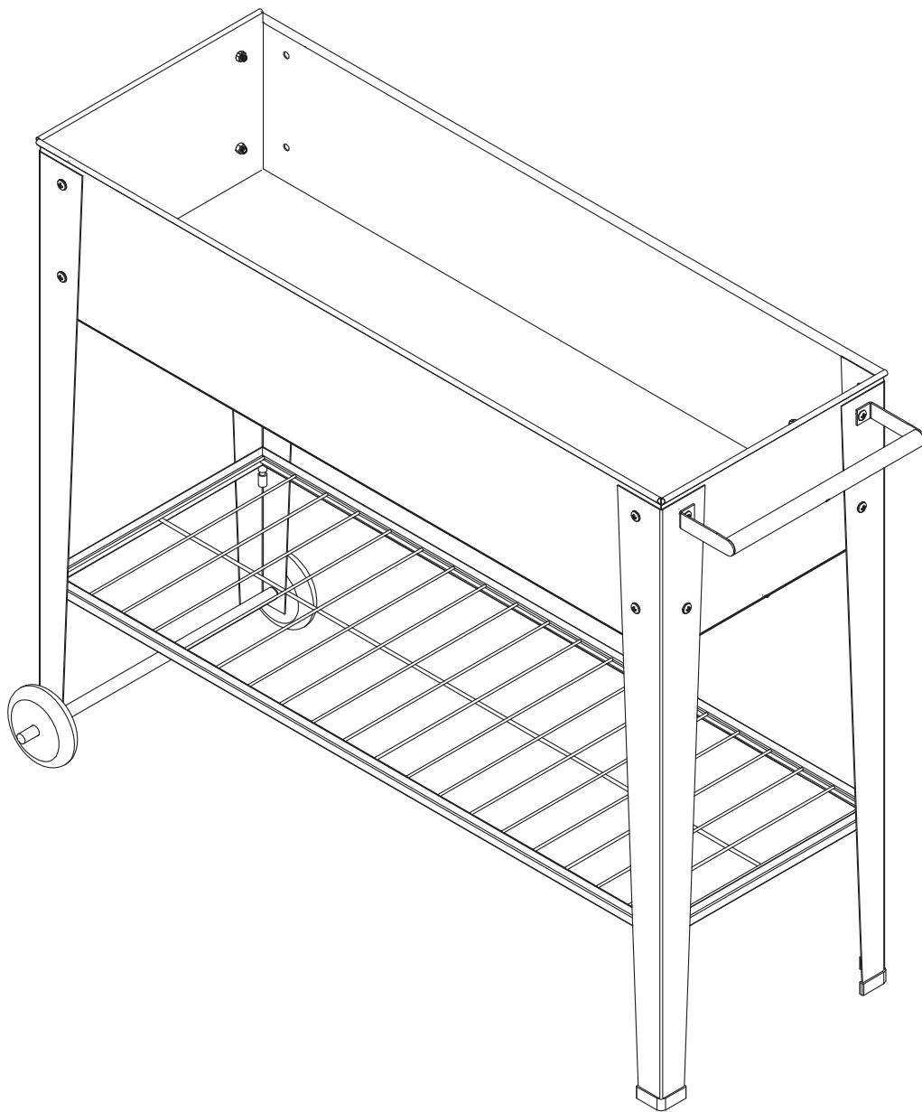
**EN** The mobile Planter Cart holds 2.7 cubic feet(70 quarts) of planting mix. The powder-coated steel Planter Cart is weather-resistant. However if the finish is nicked or scratched, use an exterior-grade metal paint to prevent rust.
