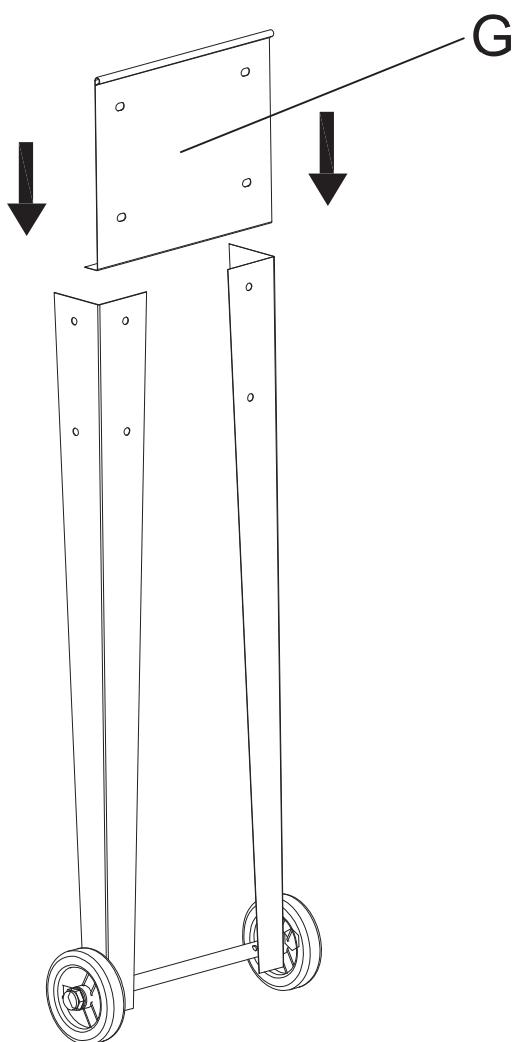
**EN\_NOTE:** The Legs should be on the out side of the planter cart with the ledge on the End Panel facing in. Insert four Bolts (L) through the lined up holes, with the heads of the Bolts on the outside and loosely attach Nuts(N)onto the ends.
