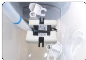
1. Remove the foam around the pump
