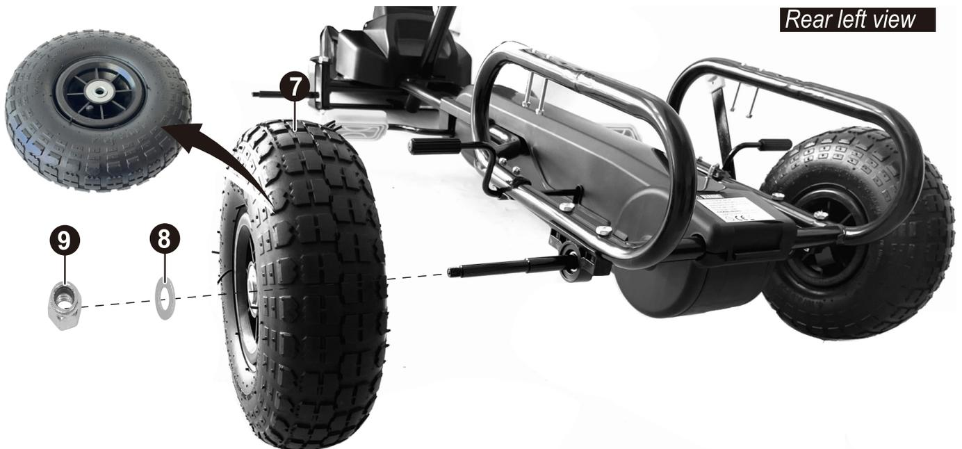
7. Slide the rear wheel into the rear axle .
