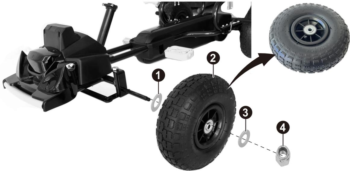
1. Slide a 12 washer onto the front axle.
