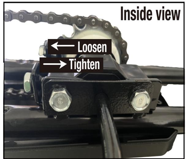
The chain must be at the correct tightness. If too tight, the bicycle will be difficult to pedal. If too loose, the chain can come off the sprockets.
