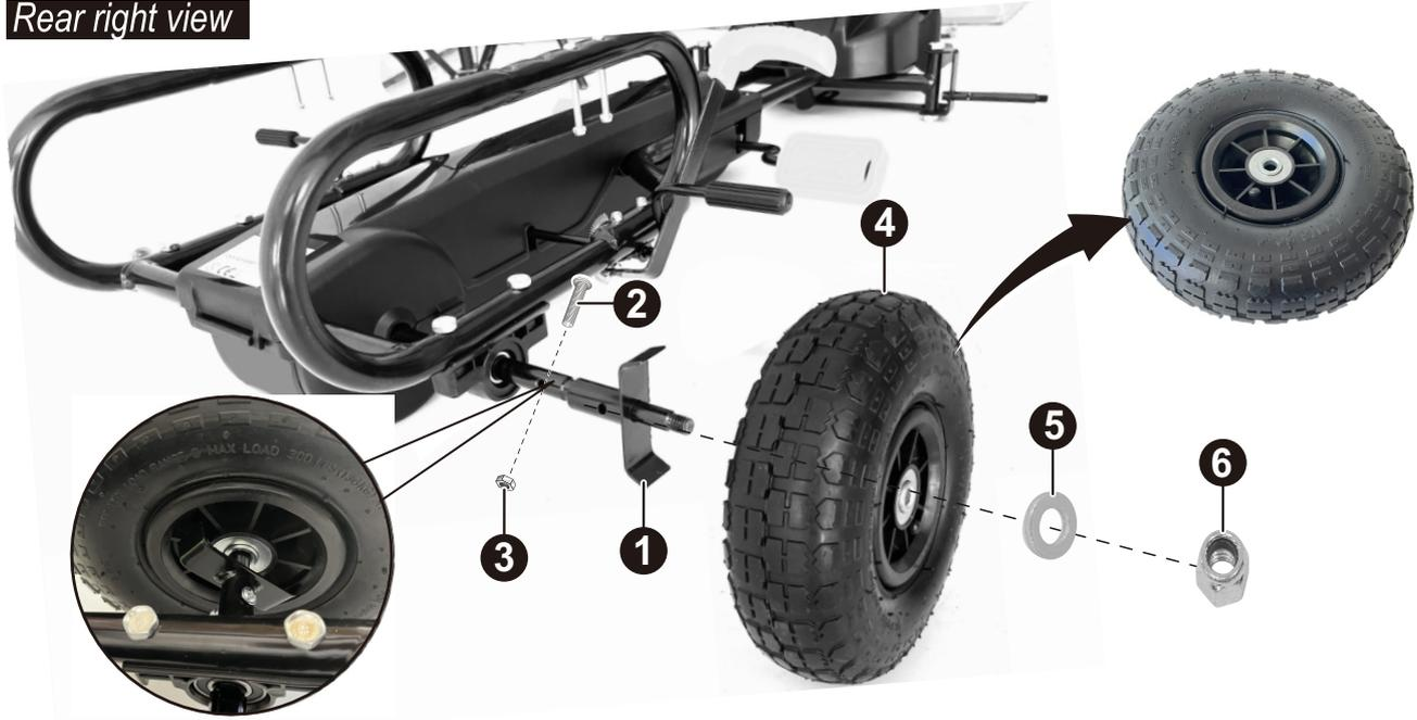
1. Slide the drive bracket into the rear axle.
