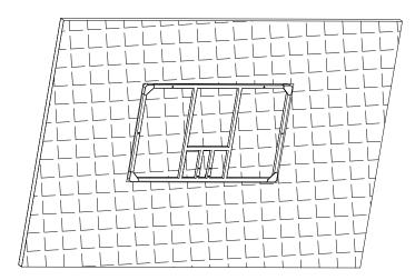
Step 3 Drill the wall/board according to the location of the backboard, and stuff the Wall plug (#1  $^{*}$  8) into the hoes.
