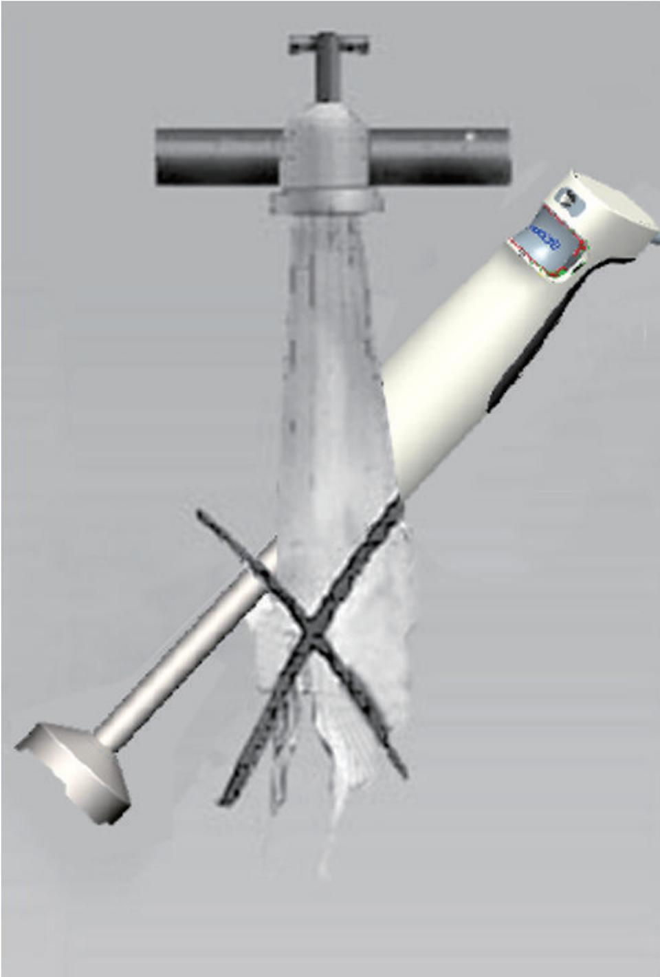
Cleaning the motor unit and chopping bowl lid only with a damp cloth only. **Do not immerse the motor unit in water!**
