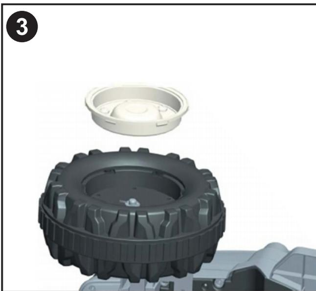
"Snap" the wheel cover into the right place, Repeat the process for the other three wheels.
