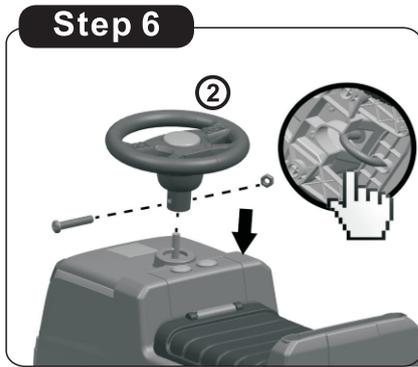
6. Loosen the bolt and nut in the steering wheel first, then place the steering wheel over the J-shaped stick, insert the bolt and tighten the nut with a screwdriver.
