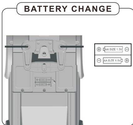
Turn over the car body, and find the battery house. Loosen the screws with a screwdriver. Put 2 AA batteries in the battery house, then tight the screw with a screwdriver.
