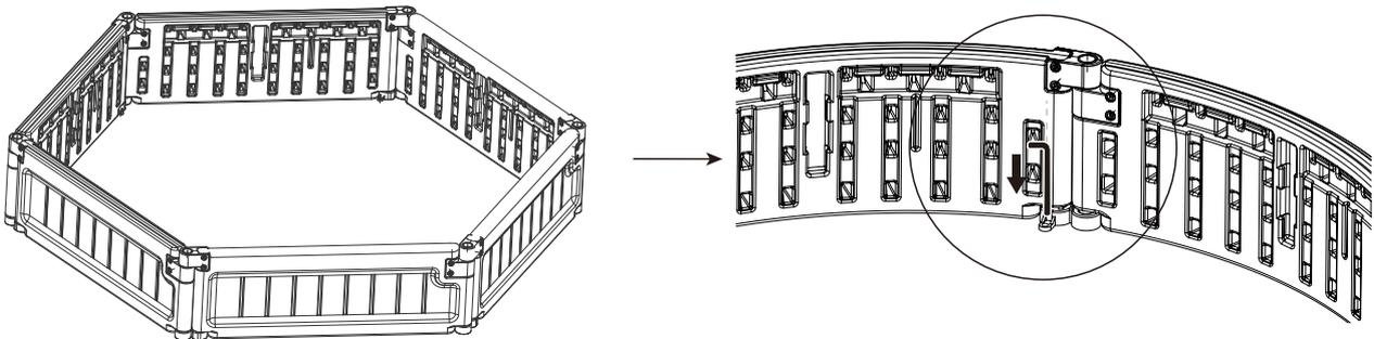
EN: Insert the "L" Pins into ground.
