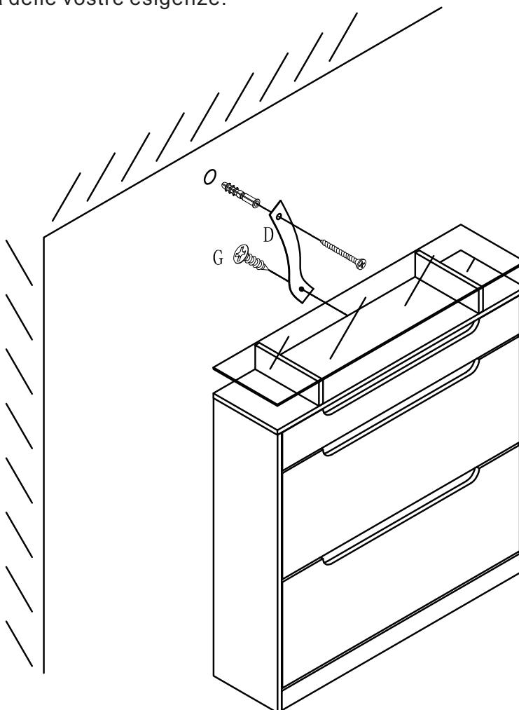
**EN** If it is a solid wall, please use expansion and self-tapping screws, if it is a wooden wall, only use self-tapping screws, please do not overtighten the screws
