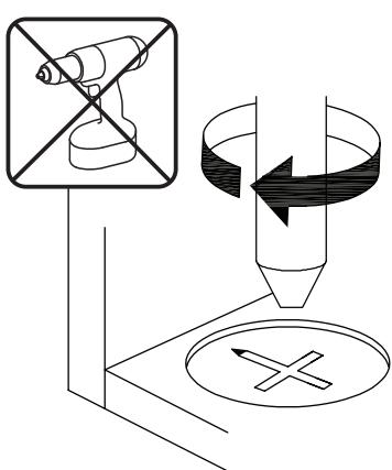
**EN**\_Turn cam lock clockwise to tighten.
