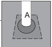
**Step2:** Combine the steel pole by 3pcs with black rubber ends, make sure the rubber ends on the center square area.
