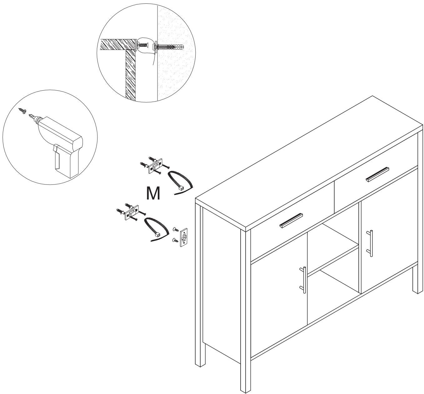
**EN** If it is a solid wall, please use expansion and self-tapping screws, if it is a wooden wall, only use self-tapping screws, please do not overtighten the screws
