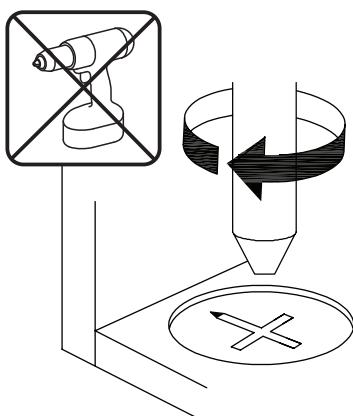
**EN**\_Turn cam lock clockwise to tighten.
