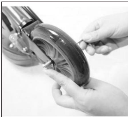
4.Use 1\*5mm hex wrench to lead and insert the axle to the hole of the front fork.
