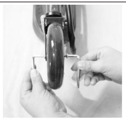
6.Use the 2\* 5mm hex wrench to insert the screw of the axle and fix with one hex wrench.
