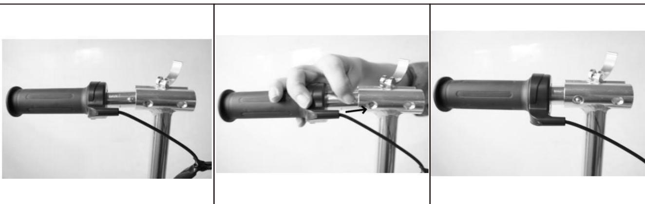
2. Insert the right handlebar of accelerator and use the finger to press the snap pin to insert and fix with the hole in the T-bar of the handlebar.
