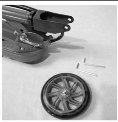
2.Take out the front wheel and the 2\*5mm hex wrench to assemble.
