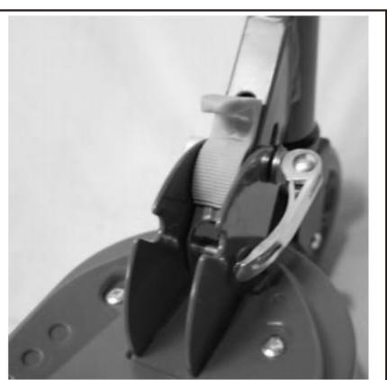
4. Twist the locker of the locking mechanism then tighten it fully and lock it tight before ride.
