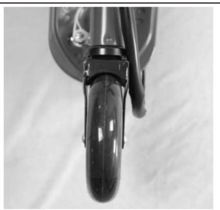
7.Twist the other hex wrench to tighten the screw with the axle and the front fork.
