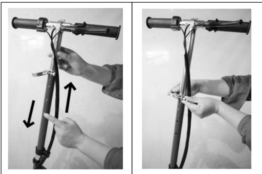
2. Press the snap pin and lift up or down the T-bar to adjust the height.
