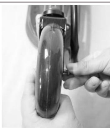
5.Insert the screw of the axle to the hole of the front fork.
