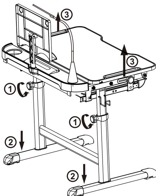
Step 1: Loosen the screws
