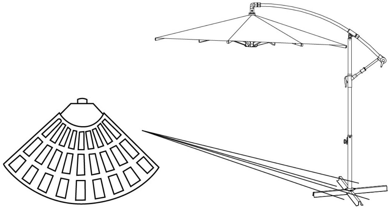
**EN** Place the water or sand filled base snug into a corner of the umbrella stand as shown in the diagram.
