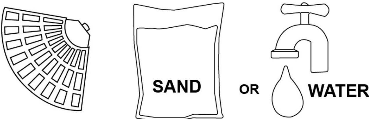
**EN** Fill the base with sand or water to increase the weight.
