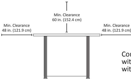
Combustible materials should not be within 60 inches of the top of the unit, or within 48 inches around the entire unit.
