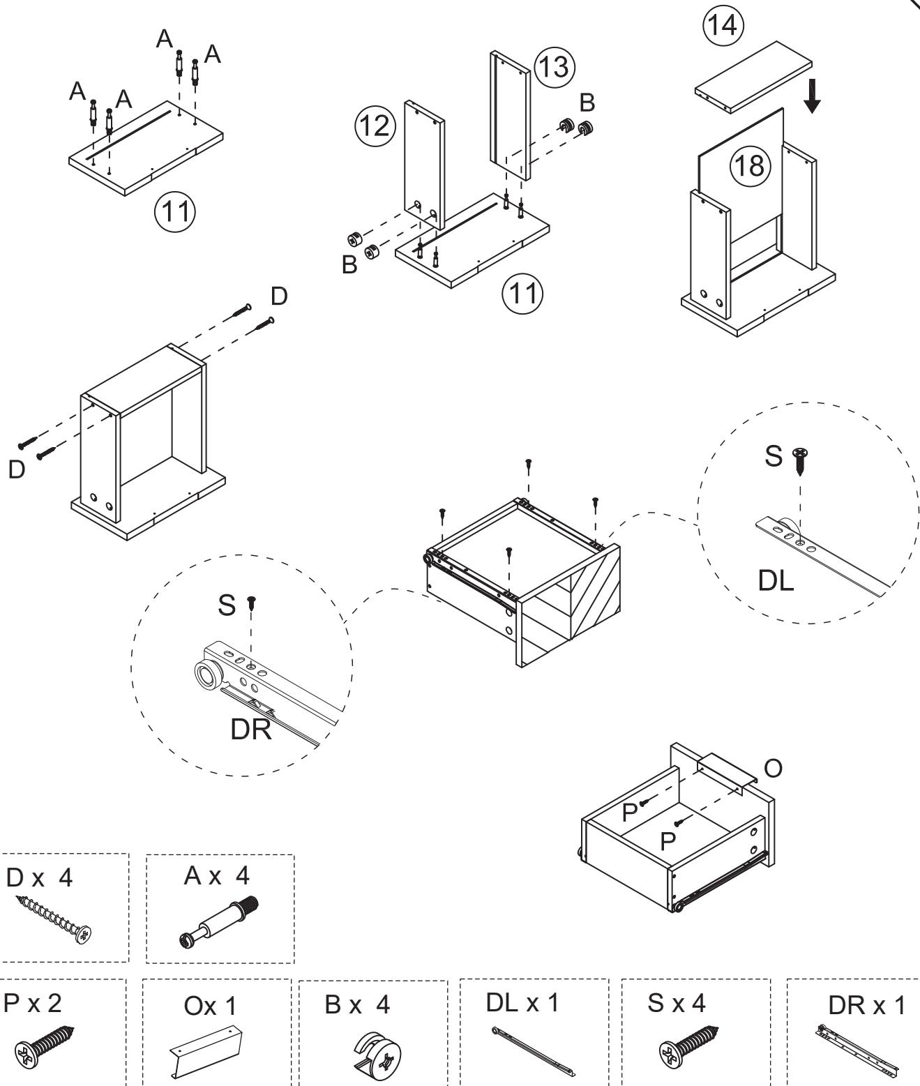
**EN** Please find the exact hole for installation, otherwise it will be misaligned. The screws on the drawer slide must be leveled , otherwise it will affect the smoothness of the drawer.
