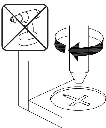
**EN**\_Turn cam lock clockwise to tighten.
