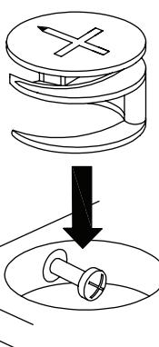
**EN**\_Quickfit head should be in the centre of the cam lock when the two panels are joined.
