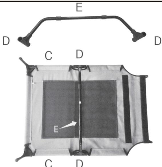
**EN** Connect the 2 center plastic junctions D to the bed support leg E as illustrated. Then insert plastic junctions D into metal pipes C.
