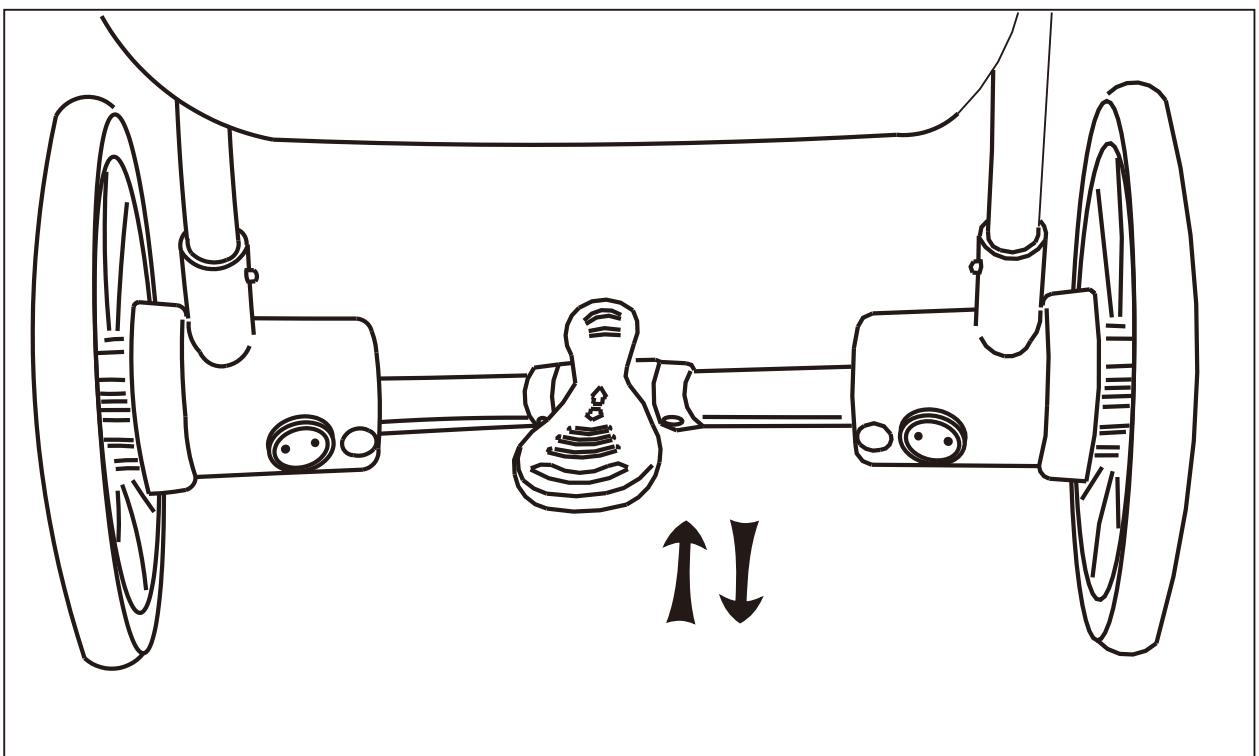
6. To step the brake pole down to stop the stroller, and lift it up to release the brake.
