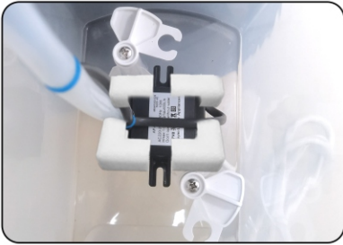
1. Remove the foam around the pump
