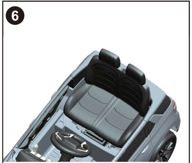
6 "Snap" the tabs on the seat into the slots of the vehicle.
