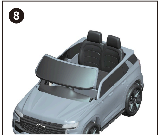
8 "Snap" the tabs on the windshield into the slots in the front top side of the vehicle.
