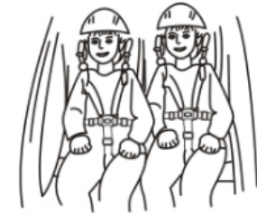
Double lock of safety belt: press the red button and then press the black one in both sides.
