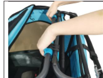
Fix the tubes with the hook
