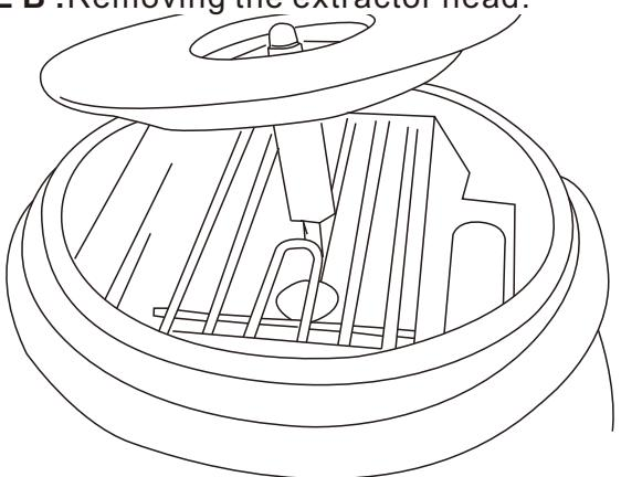
**FIGURE C :**Extractor head fits over the stem.
