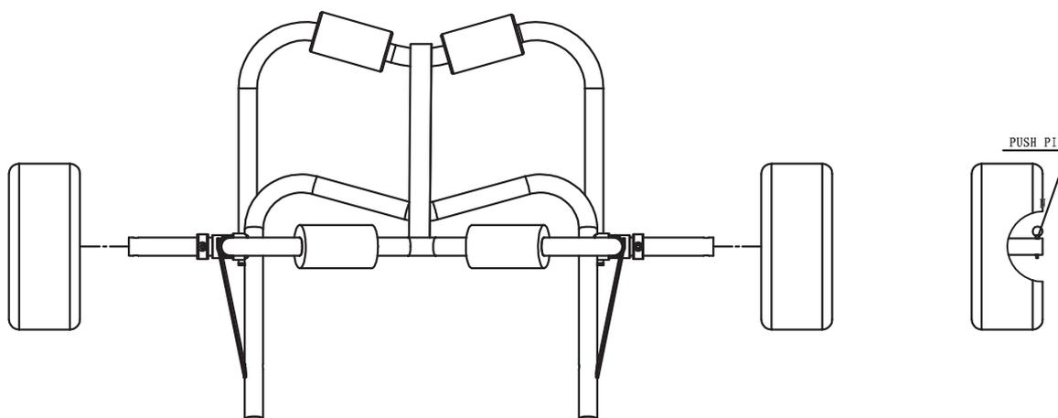
EN: Install the wheels into both ends of the cart axle, then insert the pin.
