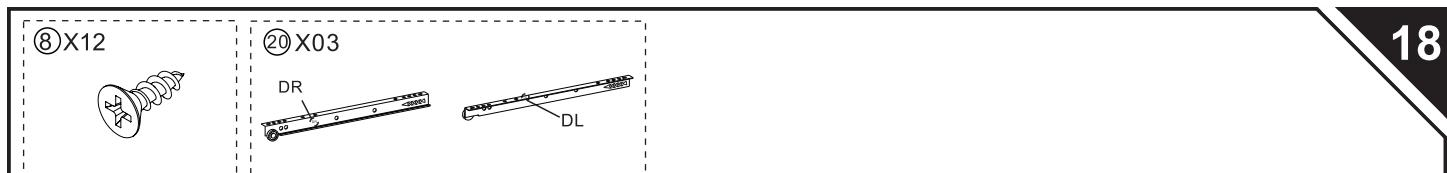
**EN** Please find the exact hole for installation, otherwise it will be misaligned. The screws on the drawer slide must be leveled , otherwise it will affect the smoothness of the drawer.
