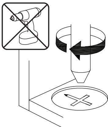
**EN**\_Turn cam lock clockwise to tighten.
