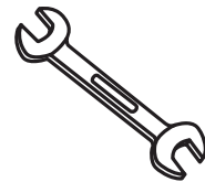
Wrench (wrenches of M17 and M14)
