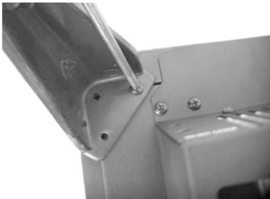
2. With use of a screwdriver, secure leg with the three screws provided (The screw is with the manual) . Repeat the above for the other three legs.
