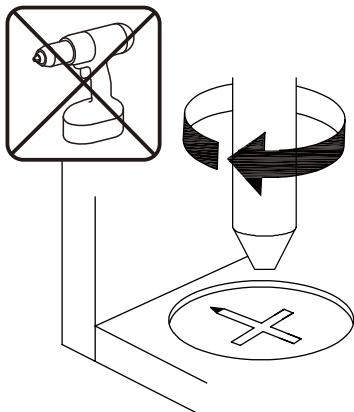
**EN**\_Turn cam lock clockwise to tighten.
