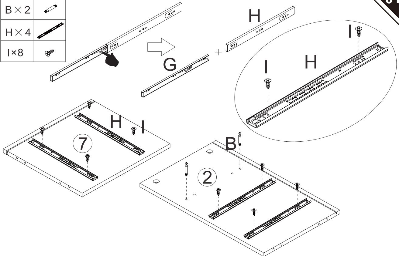
EN\_Please find the exact hole for installation, otherwise it will be misaligned. The screws on the drawer slide must be leveled , otherwise it will affect the smoothness of the d rawer.
