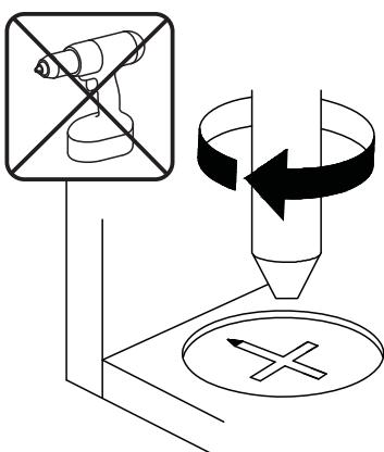
**EN**\_Turn cam lock clockwise to tighten.
