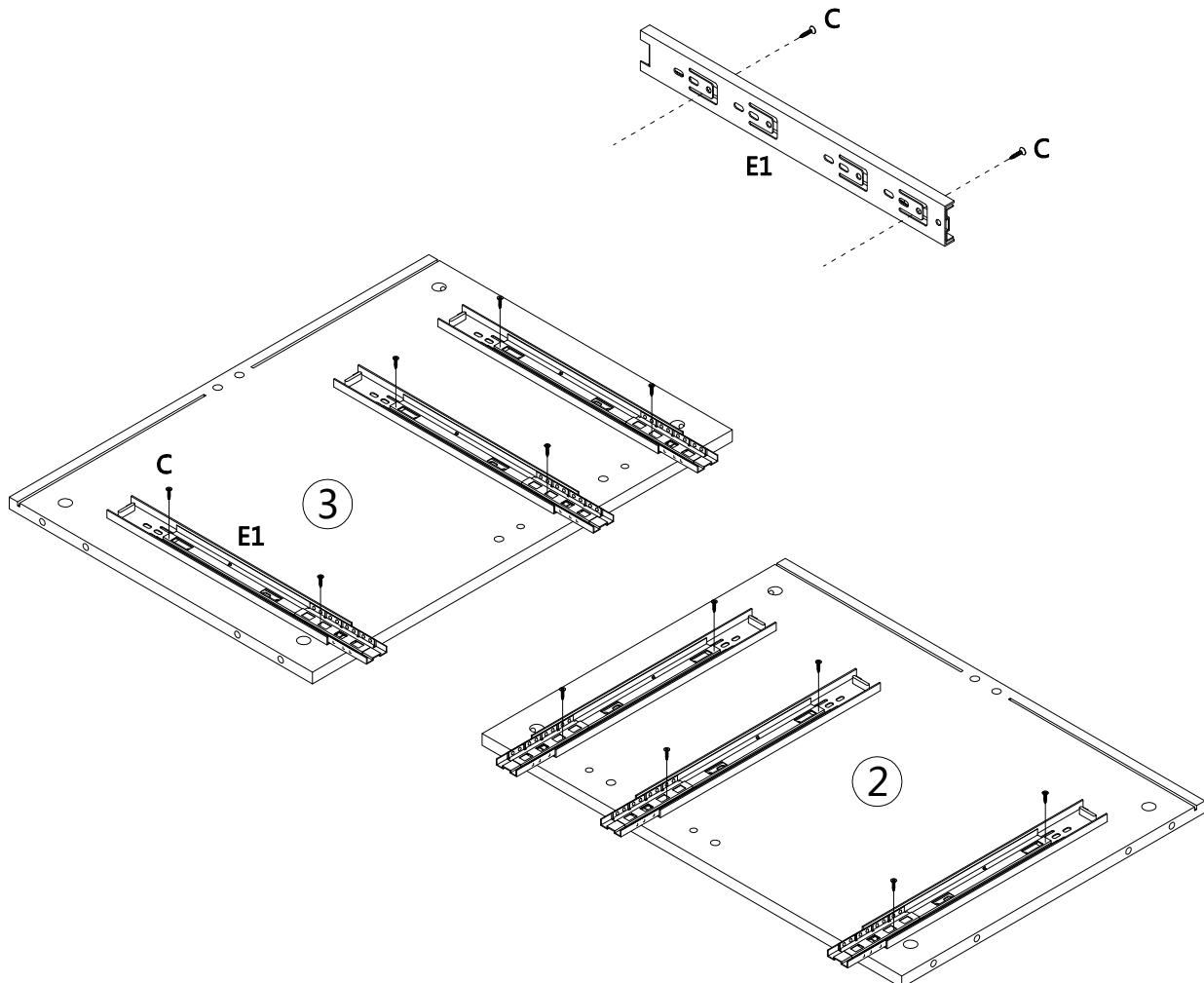
**EN** Please find the exact hole for installation, otherwise it will be misaligned. The screws on the drawer slide must be leveled , otherwise it will affect the smoothness of the d rawer.
